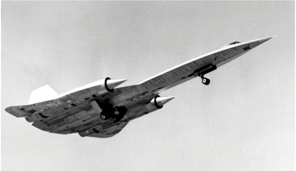
CIA developed the highly secret A-12 OXCART as the U-2's successor, intended to meet the nation's need for a very fast, high-flying reconnaissance aircraft that could avoid Soviet air defenses. (CIA photo)
